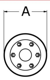
A = 208 D1 = 60 D2 = 60 L = 206 Nom. torque NM (Tkn) = 5000
